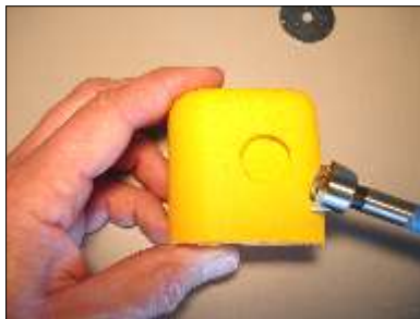
2. Drill with Forstner bit - no more than 1/2 way
