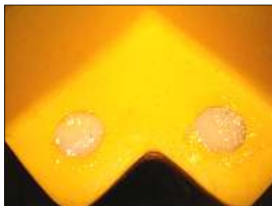
4. Fill holes with silicone
